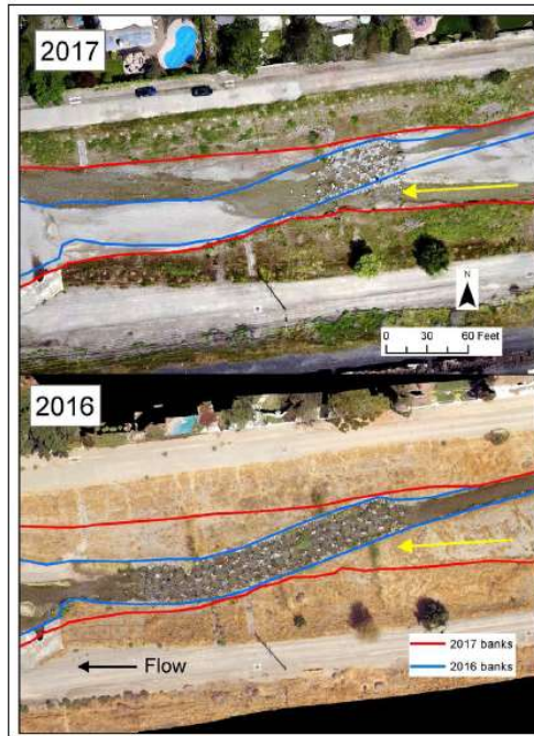
Stanley Reach Monitoring & Assessment - D160463.10 SOURCE:ESA 2017 Figure 5 Comparison between ground conditions in 2016 and 2017 Downstream Roughened Channel (Sta 25+15 to 28+15)
